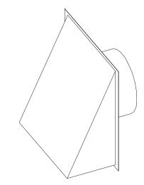
Figure 19 – Air Inlet Cap for Sidewall Termination
